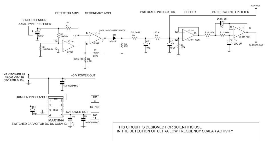
IT IS DESIGNED TO BE INTERFACED WITH A VELLEMAN VM-110 / K8055 A TO D AND PC USB INTERFACE BOARD OR OTHER A TO D UNITS AND TO USE F 3.0 CHART RECORDER SOFTWARE BY ABACOM OR OTHER SOFTWARE CHART THAT WILL WORK WITH THE A TO D CONVERTER USED.
